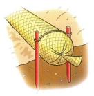
Wattles should be sufficiently overlapped to ensure effective coverage after shrinkage. Wattles come in various lengths, but the most common is 25 foot by approximately 8 inches in diameter.
